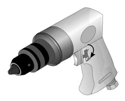
Figure 5 — Reversing the Rotation of the Drill Bit
